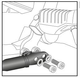
Fastening of the engine guard bottom left + right:
