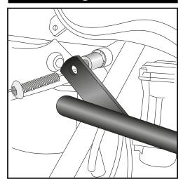
П Fastening of the engine guard top left + right: under the tank at the frame bolting with filister head screws M10 x 70 x 1,25.
